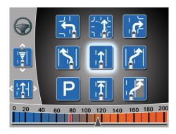
Figure 2: In this image the User Interface (UI) for maneuver based driving. The driver passes maneuver commands to the vehicle that are then translated into driving functions. The authors pointed out that it is questionable if this concept could work for every driving scenario or may it better for a context-based application (e.g. highway scenario) [3]. CHI'19 Workshop on "Looking into the Future: Weaving the Threads of Vehicle Automation", May 2019, Glasgow, UK
