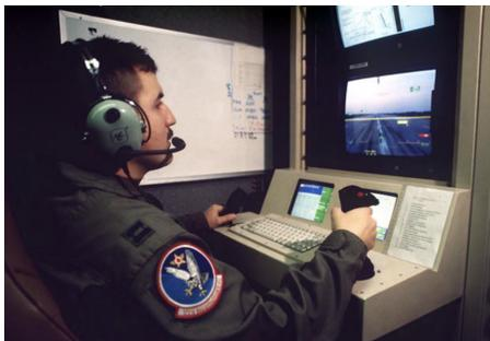
**Figure 1:** In this image an example of a direct teleoperation HMI for Unmanned Aerial Vehicles (UAV). The drone takes off and lands under manual control [1].
