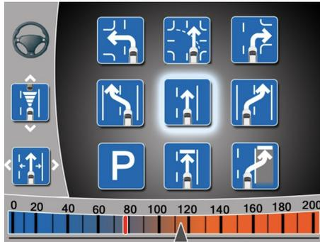
**Figure 2:** In this image the User Interface (UI) for maneuver based driving. The driver passes maneuver commands to the vehicle that are then translated into driving functions. The authors pointed out that it is questionable if this concept could work for every driving scenario or may it better for a context-based application (e.g. highway scenario) [3].
