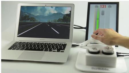
Figure 2: Scribble: a haptic interface that allows users to "draw" their way through traffic. [9].
