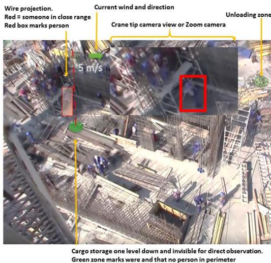
**Figure 2 Sketches on different levels of information to inform users about vehicle intentions, to present warnings, or to present more complex work-site information.**
